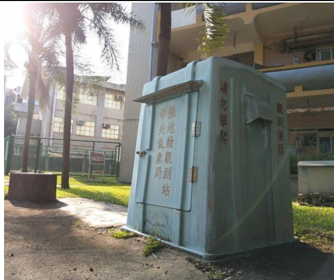
Strong motion observation station in Jin-De Campus The observation station houses the strong motion observation apparatus. The time, location, and size of an earthquake can be calculated when many stations are connected to form a seismograph network.
