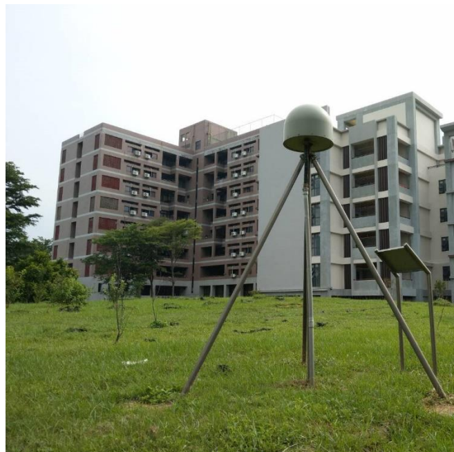
Crustal deformation observation station in Bao-Shan Campus The station continuously receives signals emitted from global satellite positioning system, and with the received signals at the same time by other stations, it can accurately calculate the station's lo-
