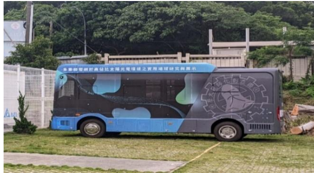
Figure 11. The 30 kW/78 kWh Pure Electric Bus.
