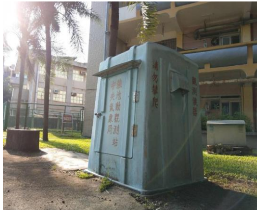
Figure 9. Strong motion observation station in Jinde Campus The observation station houses the strong motion observation apparatus. The time, location, and size of an earthquake can be calculated when many stations are connected to form a seismograph network
