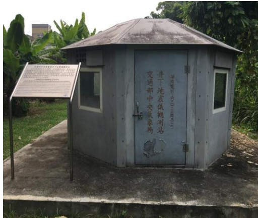
Figure 7. Underground seismograph observation station in the residential areas. The seismograph installed at a depth of 300 meters in the well can significantly reduce interference from surface noise and obtain high quality ground motion signals, improving the accuracy of seismic locating and the ability to monitor small-scale, regional earthquakes
