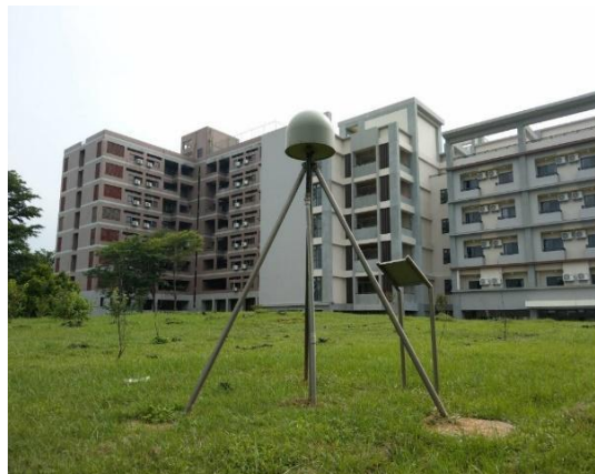
Figure 10. Crustal deformation observation station in Baoshan Campus. The station continuously receives signals emitted from the global satellite positioning system, and with the received signals at the same time by other stations, it can accurately calculate the station's location relative to other stations. Long-term observation data could reflect significant surface displacement due to major earthquakes. Also, the data on small crustal deformation occurs during earthquakes are very helpful in understanding crustal movement and earthquake potential
