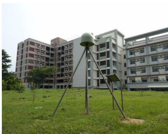
Figure 6. Crustal deformation observation station in Baoshan Campus. The station continuously receives signals emitted from the global satellite positioning system and, with the signals received simultaneously by other stations, it can accurately calculate its location relative to other stations. Long-term observation data can reflect significant surface displacement due to major earthquakes. In addition, data on small crustal deformation during earthquakes are very helpful in understanding crustal movement and earthquake potential
