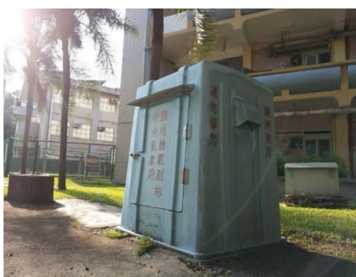
Figure 5. Strong motion observation station in Jinde Campus. The observation station houses the strong motion observation apparatus. The time, location, and size of an earthquake can be calculated when many stations are connected to form a seismograph network
