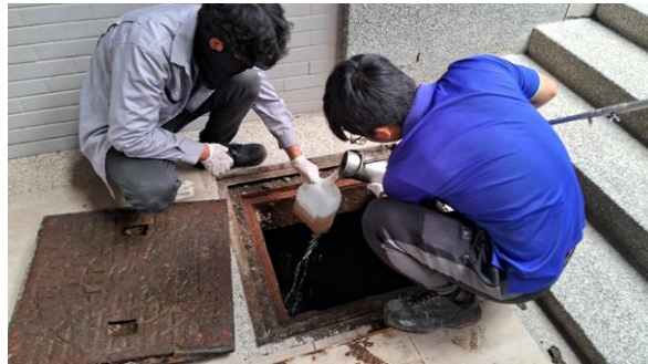
Figure 9. Workers are testing the discharged water quality treated by the sewage treatment plant on Baoshan Campus
