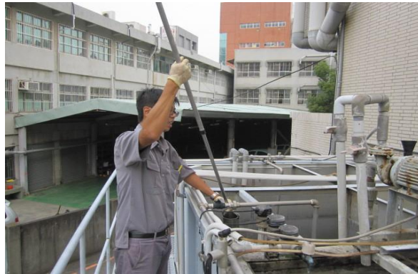
Figure 8. A worker is testing the discharged water quality treated by the sewage treatment plant on Jinde Campus
