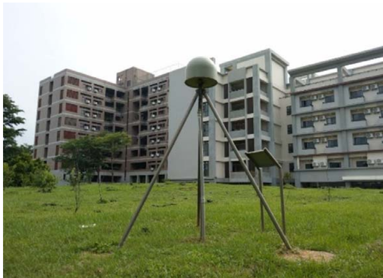
Figure 4. Crustal deformation observation station in Baoshan Campus. The station continuously receives signals emitted from the global satellite positioning system, and with the received signals at the same time by other stations, it can accurately calculate the station's location relative to other stations. Long-term observation data could reflect significant surface displacement due to major earthquakes. Also, the data on small crustal deformation occurs during earthquakes are very helpful in understanding crustal movement and earthquake potential
