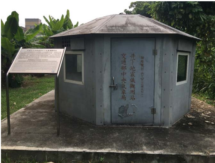
Figure 3. Underground seismograph observation station in the Family Quarters. The seismograph installed at a depth of 300 metres in the well can significantly reduce interference from surface noise and obtain high quality ground motion signals, improving the accuracy of seismic locating and the ability to monitor small-scale, regional earthquakes
