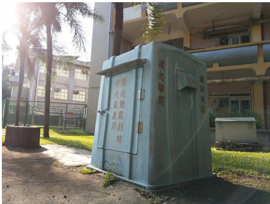
Figure 1. Strong motion observation station in Jinde Campus. The observation station houses the strong motion observation apparatus. The time, location, and size of an earthquake can be calculated when many stations are connected to form a seismograph network
