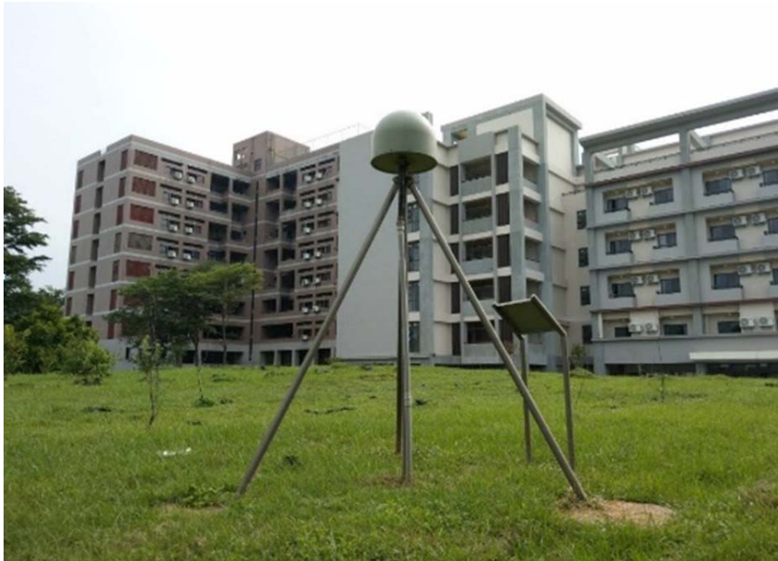
Figure 2. Crustal deformation observation station in Baoshan Campus. The station continuously receives signals emitted from the global satellite positioning system and, with the signals received simultaneously by other stations, it can accurately calculate its location relative to other stations. Long-term observation data can reflect significant surface displacement due to major earthquakes. In addition, data on small crustal deformation during earthquakes are very helpful in understanding crustal movement and earthquake potential
